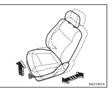
Pull up and hold the lever located under the front of the seat to unlock it. Slide the seat to where you want it and release the lever. Then try to move the seat forward or rearward to make sure the seat is locked into place.
